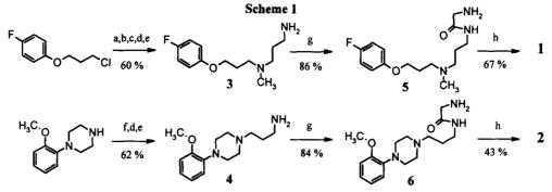
Reagents and Conditions (yields are not optimized): a) 3-amino-1-propanol,  $K_2CO_3$ , butanol, reflux; b) HCOOH, 30% HCHO, 100°C; c) SOCl<sub>2</sub>, distillation of the free base; d) NaN(CHO)<sub>2</sub>, DMF, 110°C; e) 4N HCl, 100°C; f) 1-bromo-3-chloropropane, TEA, toluene, 80°C; g) 7, CHCl<sub>3</sub>, 0°C, 1h; h) 8, CHCl<sub>3</sub>, 22°C, 8h.
